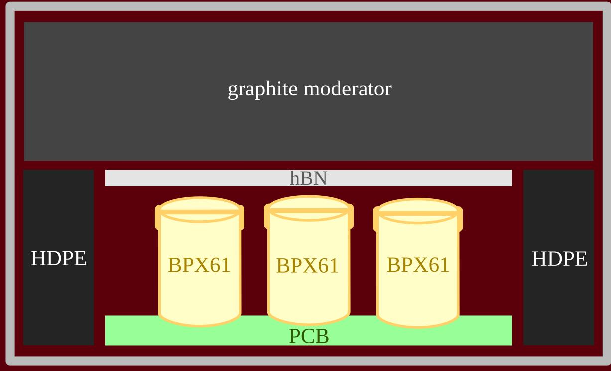
Neutron moderation is achieved using 25 mm thick graphite. The unit is made directional by shielding neutrons from non-acute angles with polyethylene. The detector is packaged in a steel tube with BNC feedthrough as EMI shield. BPX61 PIN diodes are mounted on a PCB with integrated 9V battery power supply.
