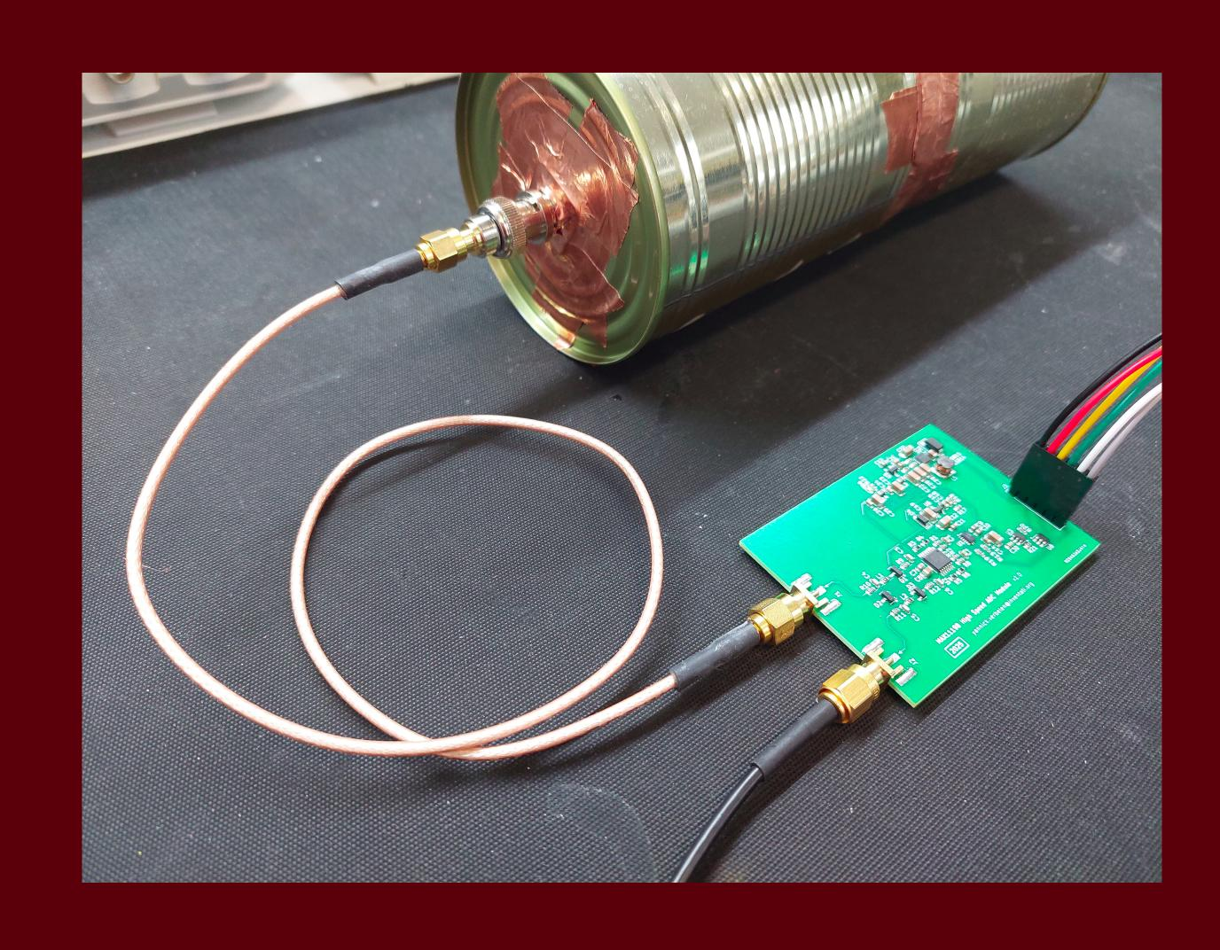
A high-speed ADC of type MAX11198 was used to acquire pulses, with a resolution of 16 bits and sampling rate of 2 MS/s. Pulses were synchronised on an external clock signal.
