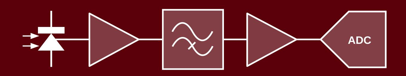
For the TIA stage, a class A cascade amplifier is composed of two low-noise 2N5088 NPN transistors [6]. A 2 M $\Omega$  feedback resistor is used for self-biasing of the TIA stage. The PIN diodes are biased via a filtered 9V supply. A 330 nF capacitor bypasses the emitter resistor to increase small signal gain.
