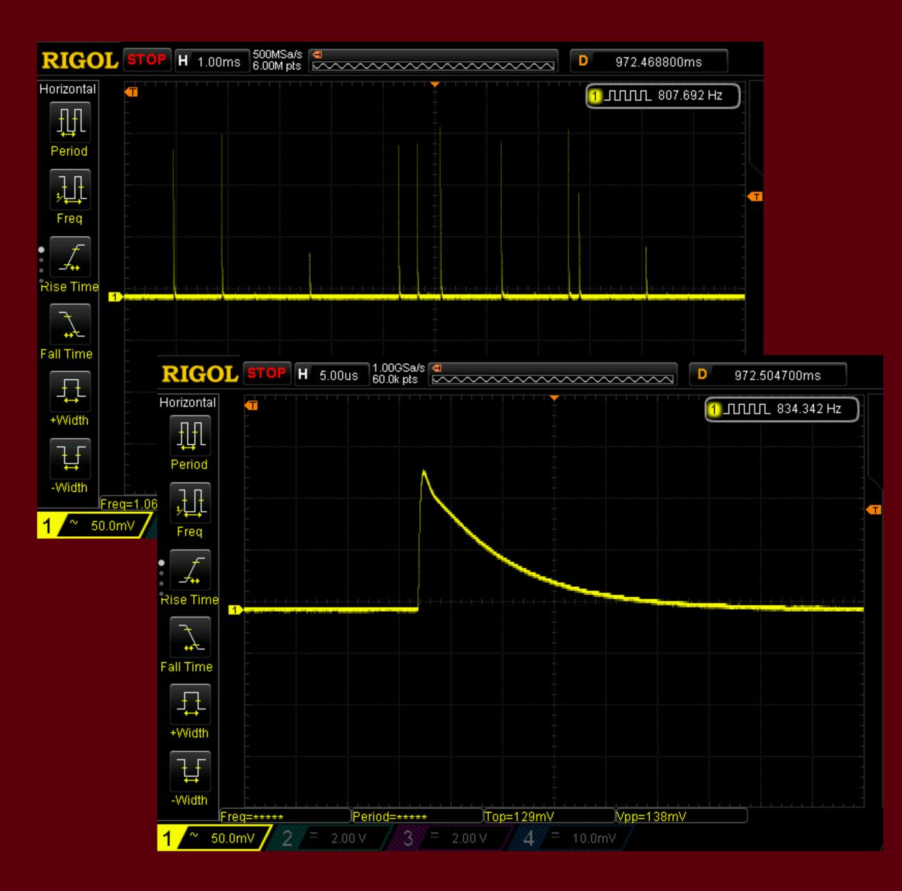
The captured pulse sequence shows alpha particles with different amplitudes captured by the BPX61 array. The period is variable due to randomness of radioactive decay. The detailed graph shows a single pulse with amplitude 130 mV and half maximum width of 15 µs. The noise is < 5 mVpp.
