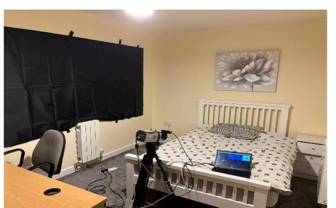
A mock house at the Berkeley Science and Technology Park was used as the test site. Two sealed Am-241 alpha sources (activities 29 kBq and 3.3 MBq) simulated criminal radioactive materials. Tests were conducted in daylight; blackout sheeting was applied to windows and door glazing to suppress ambient UV background
