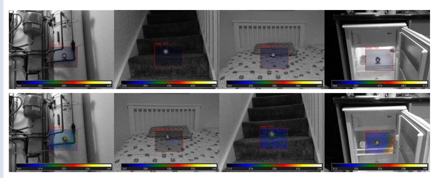
The sources were imaged in multiple rooms at 1.5 m distance. With 29 kBq, a 300 s exposure was enough; with 3.3 MBq, 10 s was sufficient. In all rooms the sources were clearly detected. A weak artefact appears in the lower-right corner of the 29 kBq image acquired in the fridge; this is likely the reflection of fluorescence light from ceiling.
