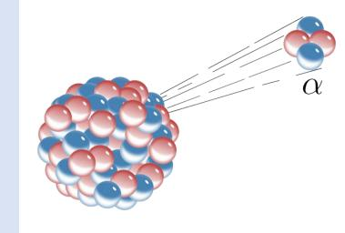
Alpha particles, consisting of two protons and two neutrons, are identical to the nucleus of a helium-4 atom. They are typically emitted through the alpha decay of heavy nuclei, where an unstable atom releases an alpha particle to transform into a different element. The travel range of alpha particles in air is generally limited to several centimetres, which makes detection challenging
