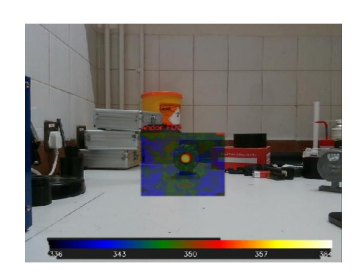
Laboratory validation has confirmed the detection of a uranium metal (surface activity: 700Bq/cm<sup>2</sup>) at 1 meter distance in one hour. The camera was also tested at an active lab in Sellafield, where it detected 2kBq/cm<sup>2</sup> alpha hot spots.
