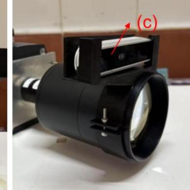
The VisionAlpha long range alpha camera ( $\approx$  3.5 kg) developed at the University of Bristol has (a) ultra-sensitive, deep-cooled CCD. (b) high-aperture lens system and high blocking rate ambient light filtering system. F-number around 0.74 and angular field of view  $\sim$  16°. (c) A co-aligned depth/RGB module provides an immediate visual context for rapid localisation of alpha-emitting areas. It has been tested in an active lab in Sellafield and is currently at TRL7
